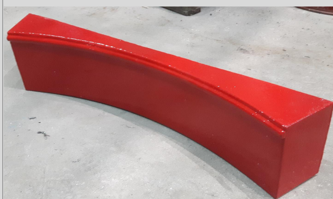
Modular polystyrene formwork of a test segment
