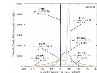
Figure 6: Comparison of repeatability and accuracy of DIC, FOS and strain gauges
