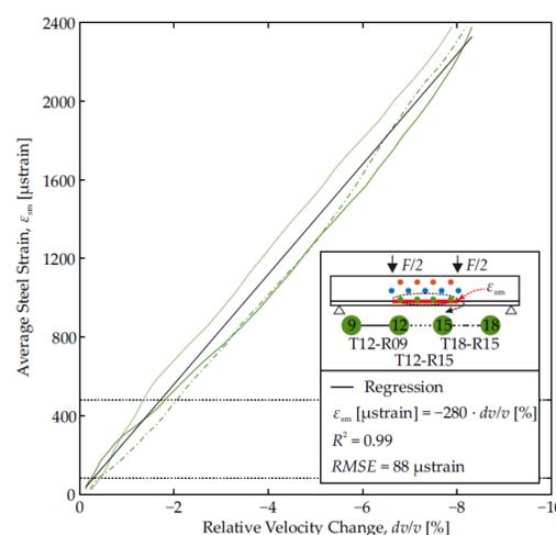
Figure 9: Strong correlation of the average steel strain and the relative velocity change
