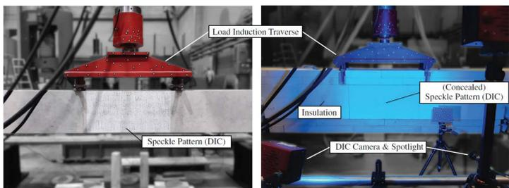
Figure 7: Photos of beams during mechanical and thermo-mechanical testing
