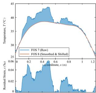
Figure 8: Sound separation of coupled effects in fiber optic measurements
