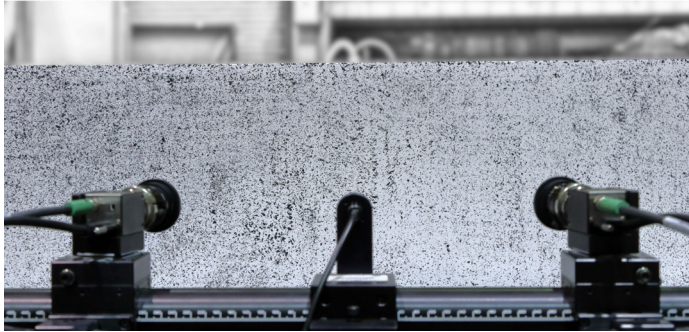
Figure 2.11: Speckle pattern and cameras for DIC strain measurements
